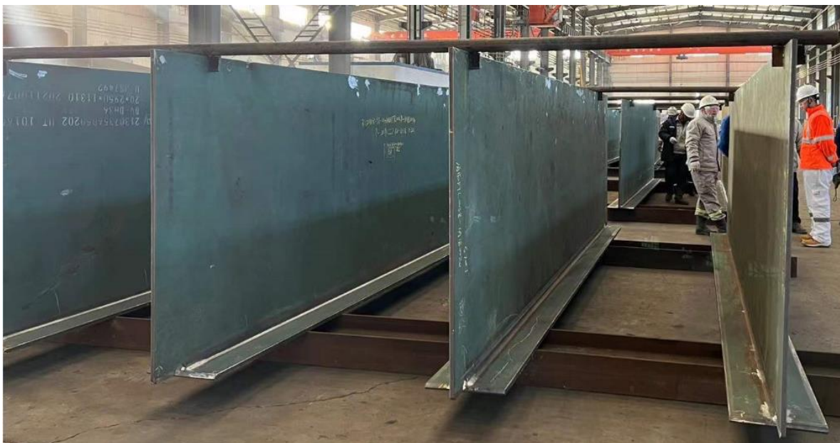
图5 PG梁防倾措施 a Fig.5 PG overturn-preventing a
